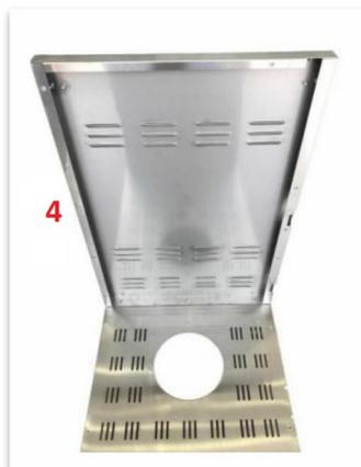
STEP-4: Attach Bottom Back Panel (#5) to the Side Panels (#3 & 4) by using 6 sets M5x12 screw with captive washer and then to the Bottom Panel (#2) by using 3 sets M5x12 screw with captive washer.
