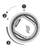
**Note:** If the magnet in the knob is disconnected, the indicator light will be orange. If the knob arrow is facing UP, gas is not flowing.
