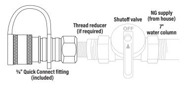
**STEP 03** Connect your appliance to the natural gas supply from the source by removing the dust covers and making sure both fittings are free from any debris. 1 Pull the locking collar back on the fitting and 2 push the male Quick Connect fitting all the way inside and then release the locking collar.
