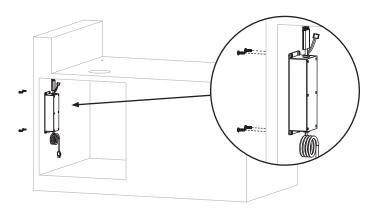
STEP 06 With the help of another person, direct the hose and electric wires through the cabinet hole and place the griddle body on top of your cabinet.
