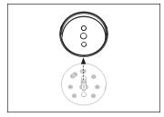
STEP 04 Lift out the knob PCB, and disconnect the wire from the back of the knob PCB.
