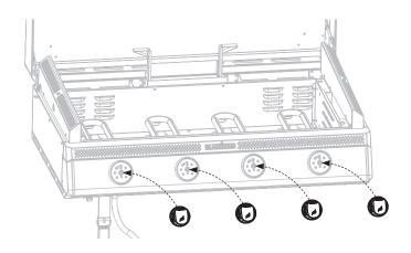
**STEP 04** Remove the four (4) protective washers from the griddle foot pins. **With the help of another person**, place the griddle top onto the griddle body by aligning the four foot pins to the holes on top of
