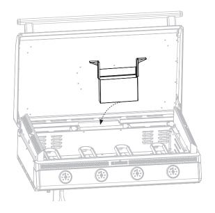
**STEP 03** Install the four (4) control knobs by pushing them into place in the OFF position.
