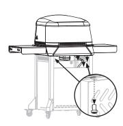
STEP 02 Thread the four M6x14 black screws back into the oven body.
