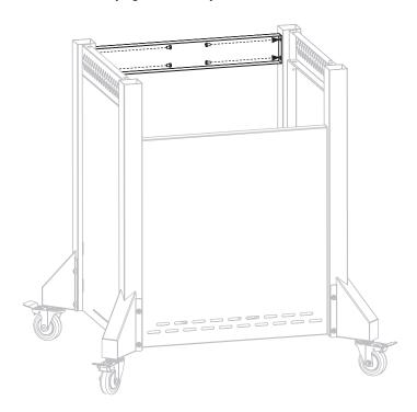
**STEP 14** Use two (2) M6x12 screws [b.] to attach the limiter to the left cart panel and the cart base.
